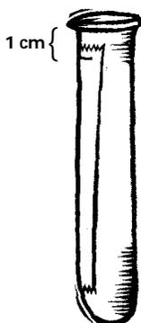
**4** Wet a small piece of steel wool, about the size of a quarter. Press the steel wool into the bottom of one of the test tubes. Use a pencil to wedge it in tightly.
